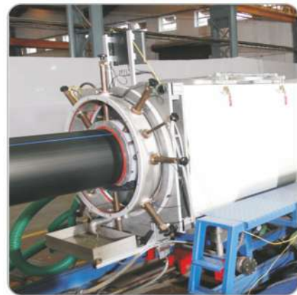
VST 630 with optional feature of ultrasonic sensor to measure pipe wall thickness
